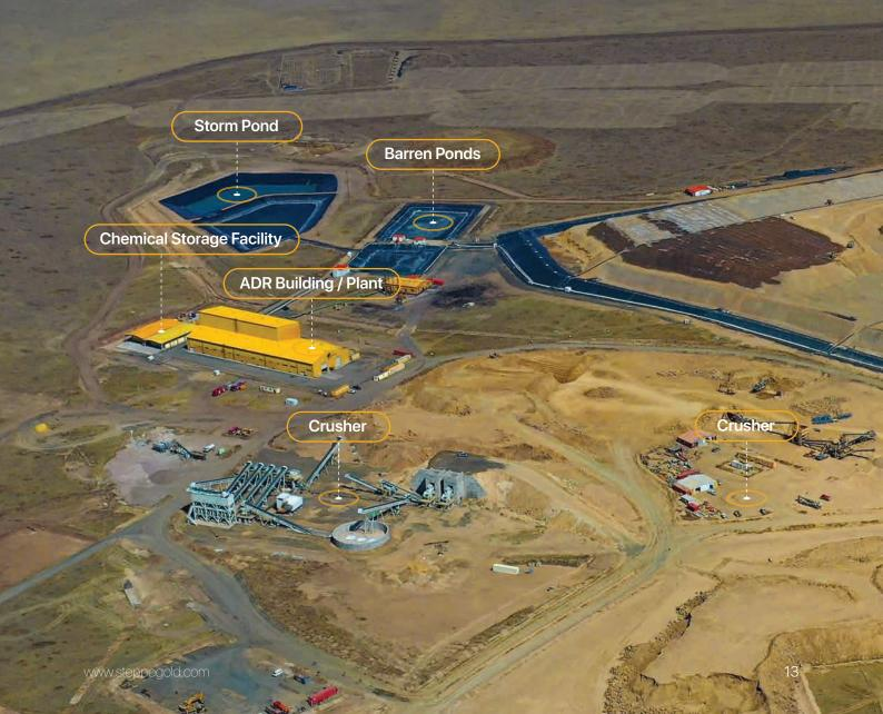
With Phase 1 oxide production ongoing, the focus now shifts to Phase 2 fresh rock expansion. Phase 2 Expansion will boost gold production and generate marketable concentrates of lead, zinc, and pyrite through the development of underlying fresh rock ores including the establishment of a flotation plant.
