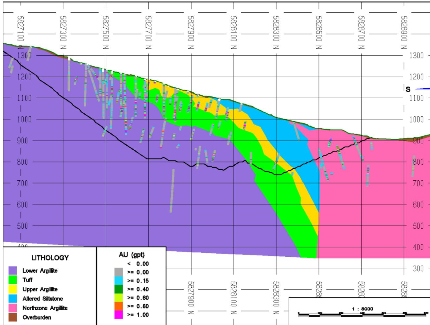
Figure 10-15 Section East 604325 looking West with Drill Grades (+/- 10 m from section) Relative to lithology and Resource Pit Shell
