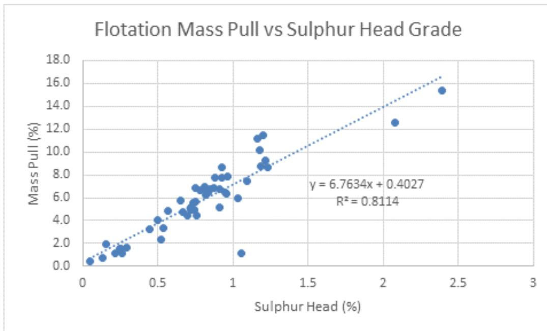
Figure 13-15 Sulphur Head Grade and Flotation Mass Pull Relationship at 10 g/t Au grade concentrate
