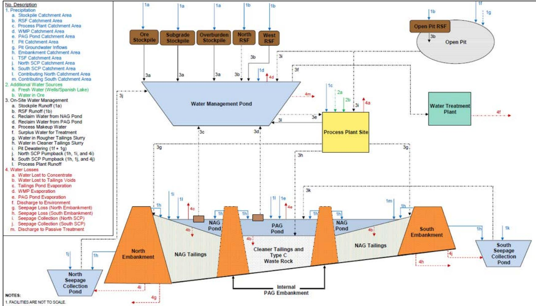
Figure 18-4 Year 1 through 14 Water Balance Schematic
