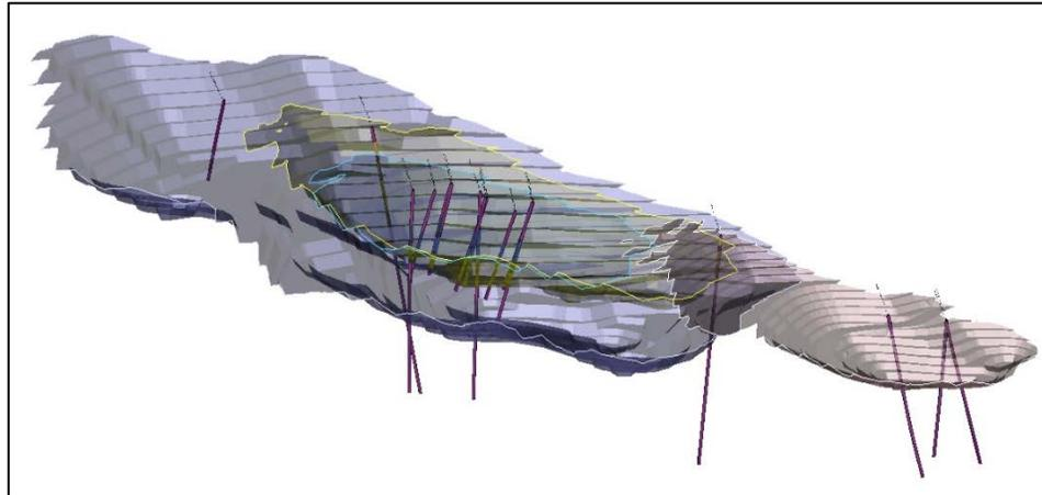
Figure 13-2 Cross-section of the Open Pit Showing the Drillholes for Metallurgical Testwork
