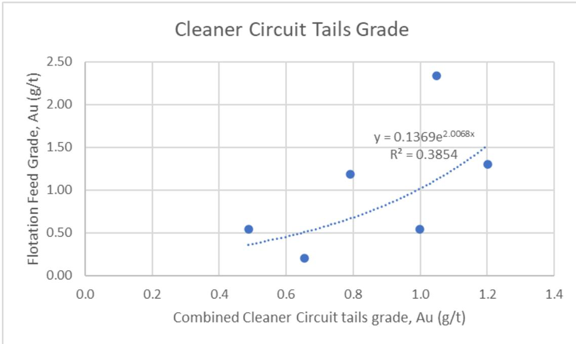
**Figure 13-16 Flotation cleaner circuit tailings grade as a function of flotation feed grade**
