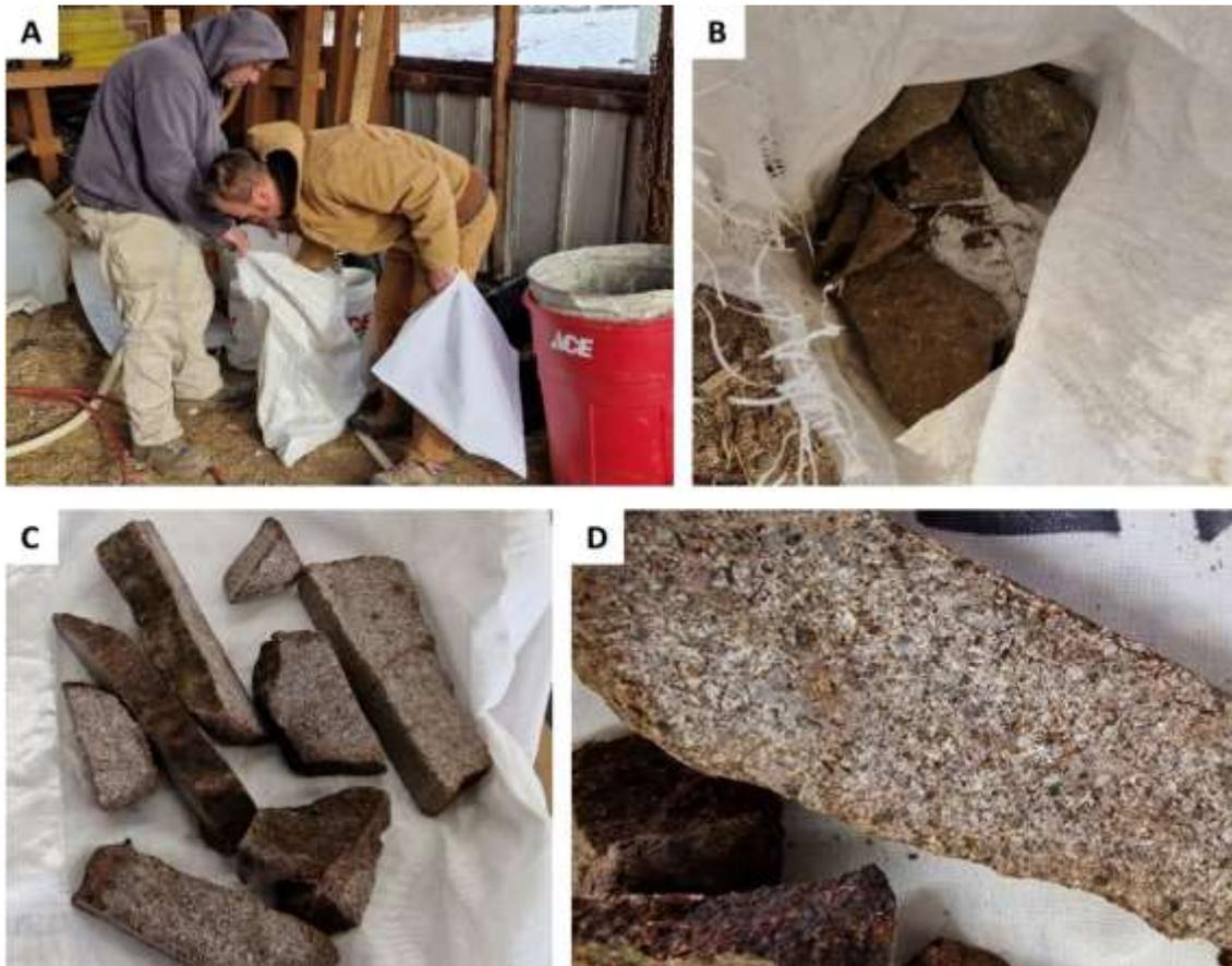
A) Challis Tuff sample selection and preparation by field/core shed lab technician, Clayton Campbell and supervising Principal Geologist, Dan Pace - B) Bulk Challis Tuff from the Property's outcrop; C)-D) Prepared blank samples made of Challis Tuff
