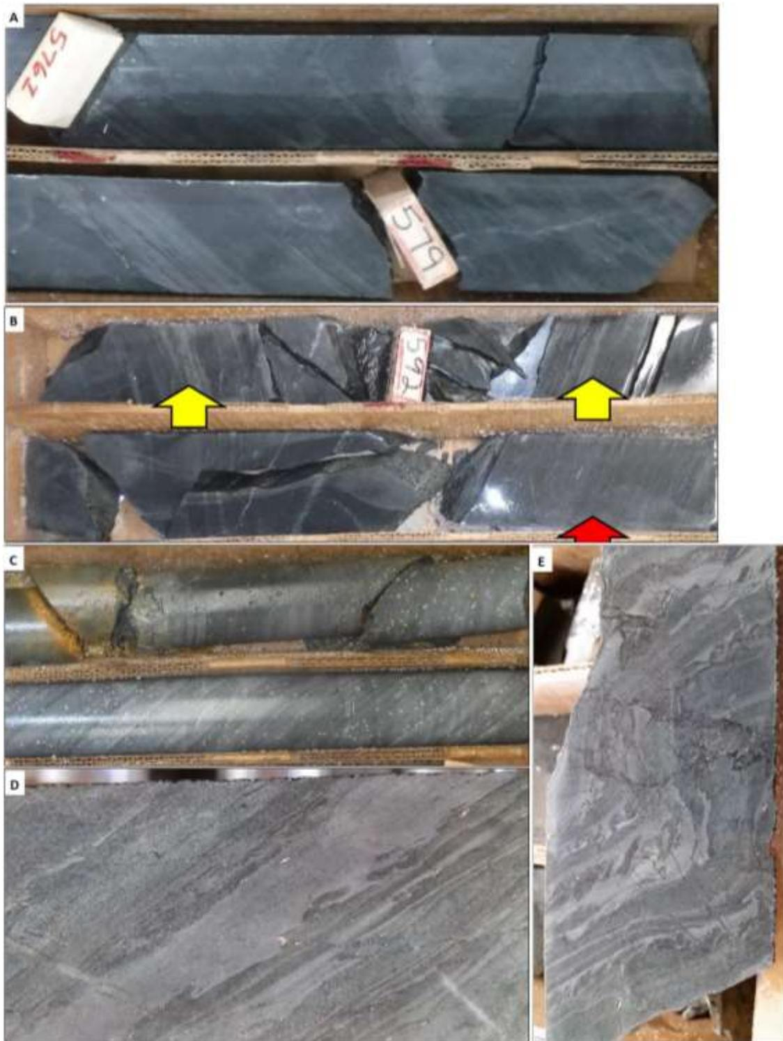
A) Siltite (SLTT); B) Quartzite (QTZT): thin (yellow arrow) and thicker (>5cm; red arrow) coarse inter-beds of quartzite are prominent within siltite; C) Bleached Siderite Unit (BSU); D) Rhythmically Bedded Unit (RBU); E) Siltite-Quartzite Disrupted Unit (SQD)
