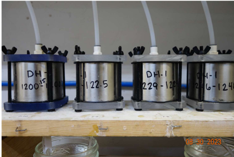
Figure 6. Rapid Brine Release (RBR) sample testing configuration
