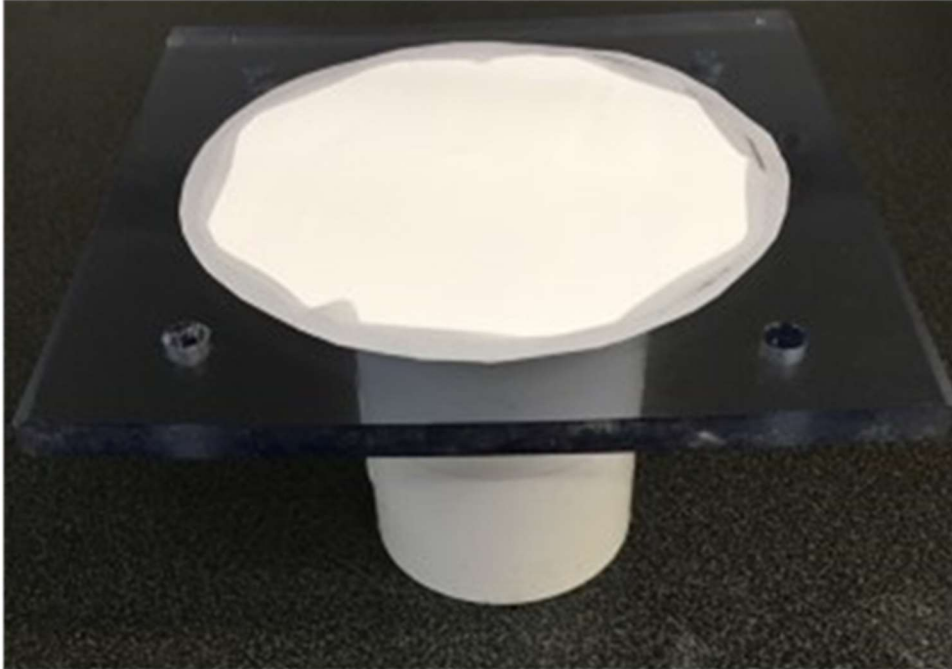
Figure 4. Pre-wetted micro-pore membrane on the bottom PVC cap
