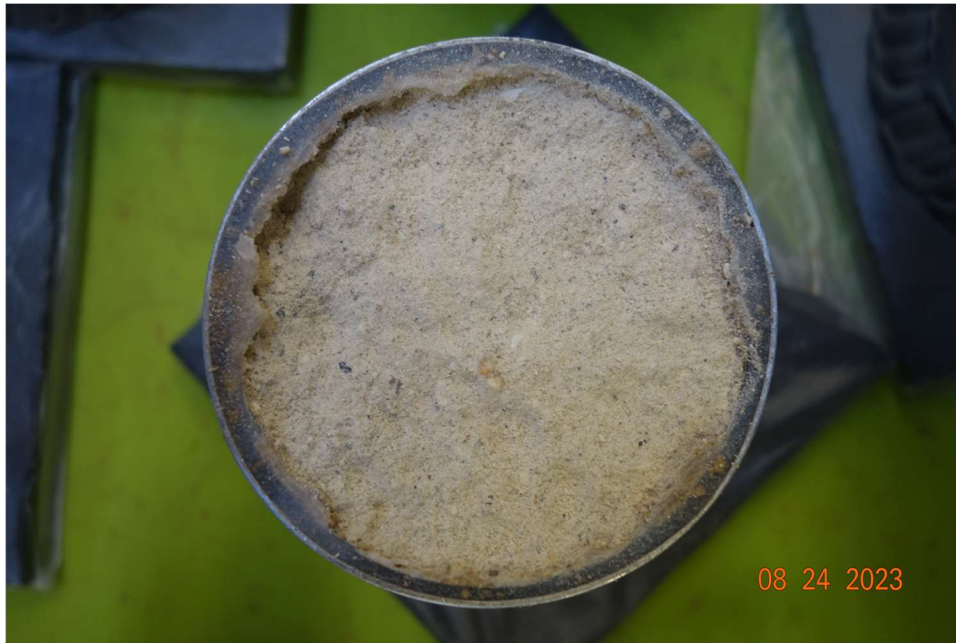
Figure 3. Silicone packing method for consolidated cores; sample DH-1 1200.15-1200.75
